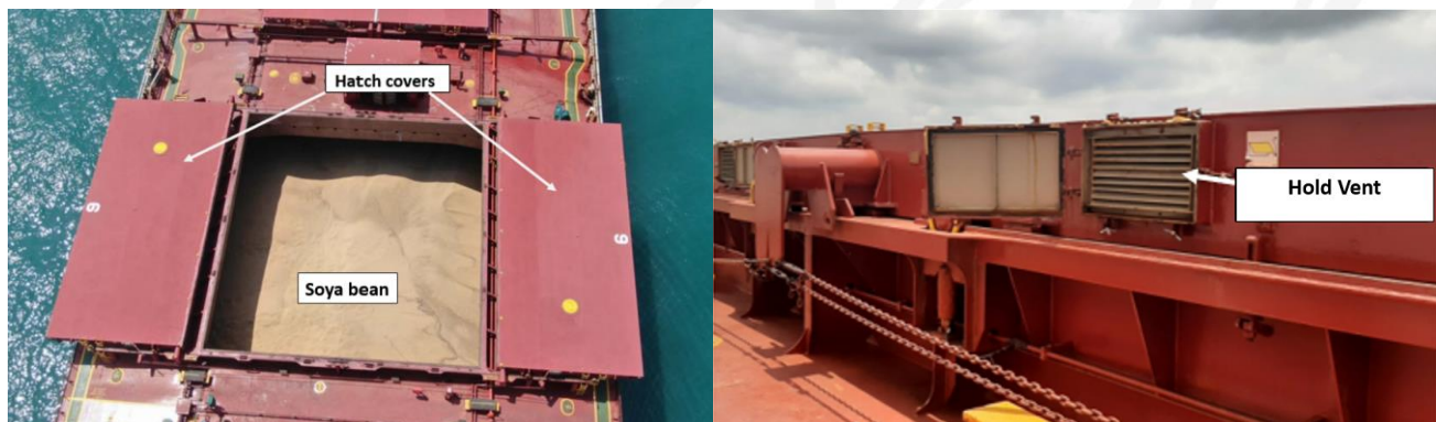
Figure 1. Aerial view of No.6 cargo hold and hold vent
