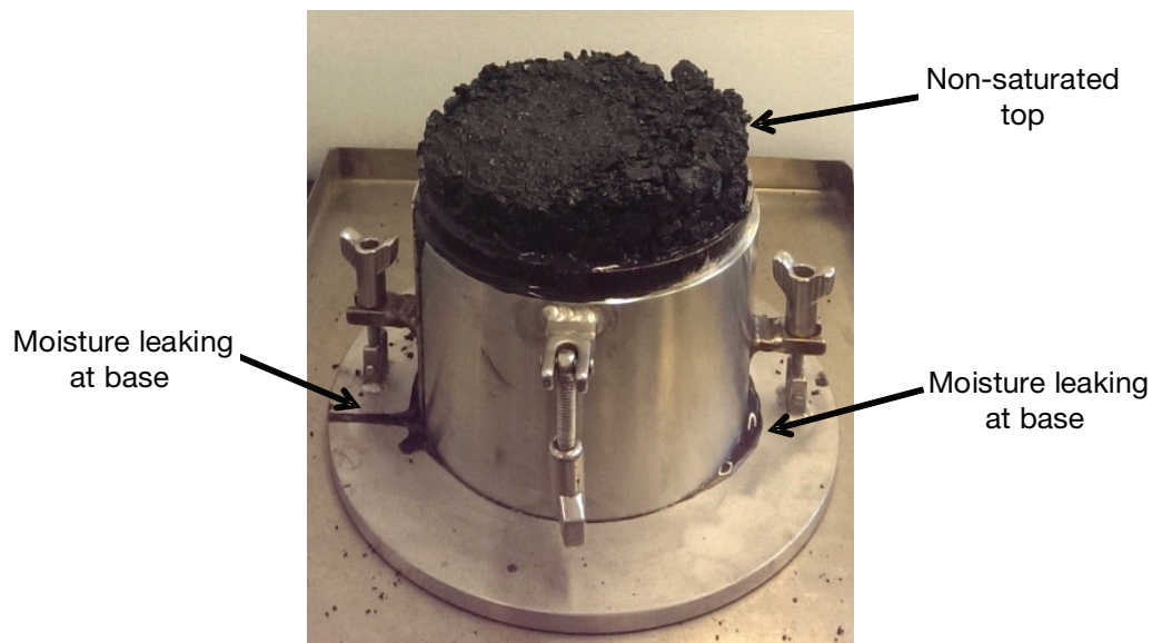
Figure 1.5.5.3.4.2 – Test showing water leakage from the base of the cylindrical mould indicating moisture migration
