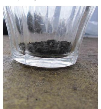
2. Carefully add sulphuric acid, covering the cargo sample to a depth of 3 to 5 cms.
