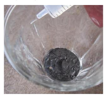
3. Check whether the sulphuric acid causes bubbles (hydrogen gas) to rise from the cargo sample.
