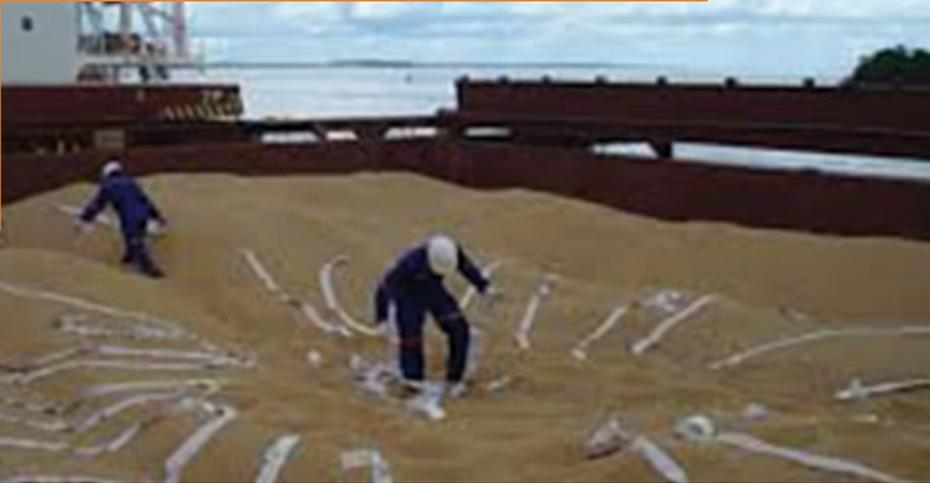
As noted earlier, the presence of free water in contact with aluminium phosphide tablets will speed up the reaction causing higher temperatures and the production of more phosphine gas, heightening the possibility of a flammable atmosphere being formed in the hold. The cargo surface must therefore be kept dry, protected from precipitation during loading and, it should be considered that sweat may form on the cargo or on hold steelwork while the holds are sealed whilst fumigation is in progress.
