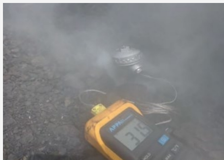
Coal on a barge measured to be below 55°C but clearly self-heating as evidenced the smoke /steam
