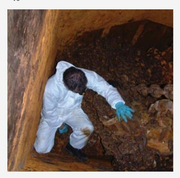
Three crewmembers died after entering this chain locker where heavy rusting had reduced the oxygen content to less than 10%
