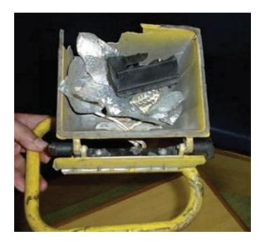
This non-intrinsically safe halogen lamp was placed just inside the door of a boiler steam drum shortly after it was opened for inspection following a chemical clean. The tank atmosphere exploded causing fatal injuries to one of the personnel outside the steam drum door.
