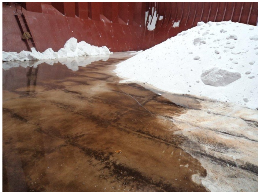
This fertilizer cargo was damaged by sea water migrating from an adjacent holed ballast tank
