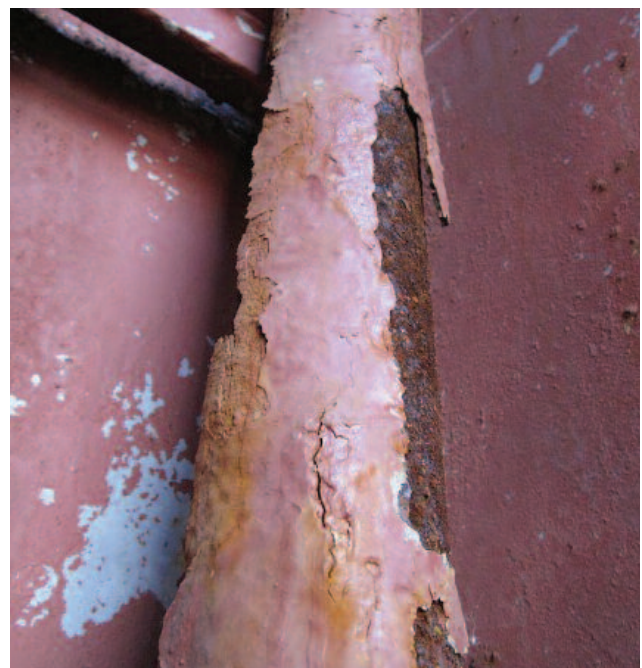
Hold components and pipework heavily corroded.
