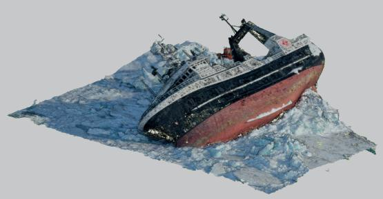
This is 3D model of the grounded fishing vessel 'Northguider' created using photogrammetry from a drone
