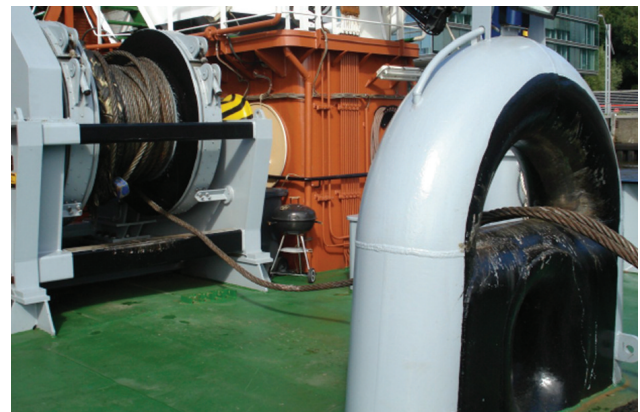
Heavy duty tow wire lead near the stern on a harbour tug fitted with 3 azimuthing propellers in Kort Nozzles; 2 forward and 1 aft
