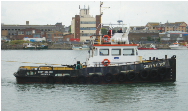
Conventional tugs and towing vessels are at greater risk of girting
