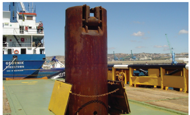
A towing pod on an ocean going tug
