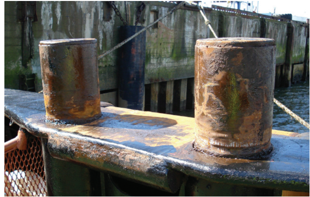
Towing pins on the aft bulwark of an ocean going tug
