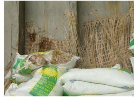
Bagged Rice damaged as a result of ship sweat when in contact with Shell Plating in a Cargo Hold
